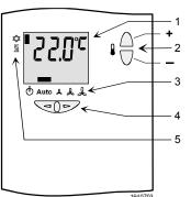
Display of actual room temperature or adjustment value, and bar indicating sequence (heating/cooling), operating mode and fan speed.
