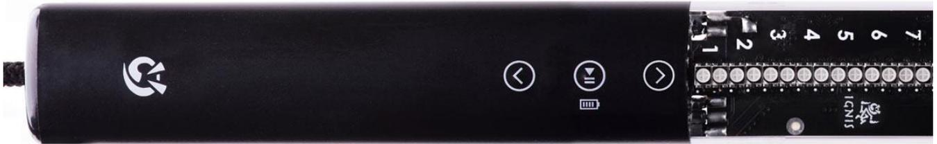
To switch poi on/off press and hold central button
