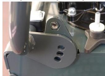
Unscrew the cross-headed screw. The desired height can be chosen using the three bore holes provided. Screw in the cross-headed screw at the desired height.
