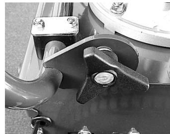
Position the swivel bracket for the sweeping brushes in the centre of the machine. Unscrew the cross-headed screw. Now slowly fold down the steering bar towards the motor cover. While doing so, hold the Bowden cables at the right and left of the motor block.
