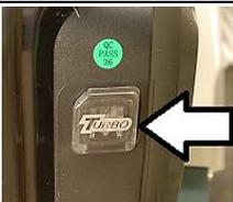
This LED lamp indicates the power increase to 3300 revolutions. If more power is required for the sweeping work, the motor automatically switches to the power setting.
