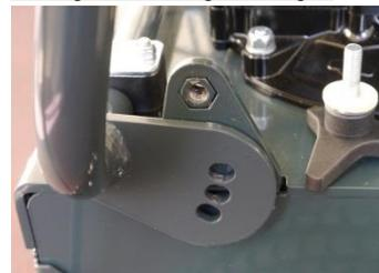
Unscrew the cross-headed screw. The desired height can be chosen using the three bore holes provided. Screw in the cross-headed screw at the desired height.
