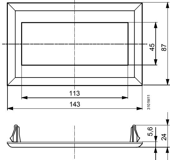
Panel cutout if controller shall be wired prior to mounting:
