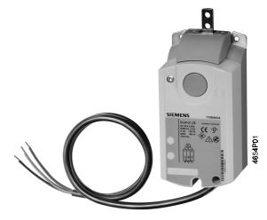
Electric motor-driven linear actuators for three-position control, nominal linear force 125 / 250 N, nominal travel 60 mm, AC 24 V or AC 230 V operating voltage, pre-wired with connecting cables of 0.9 m.
