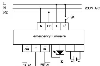
The emergency luminaire with installed ECS110 addressing module (for a central monitoring system)
