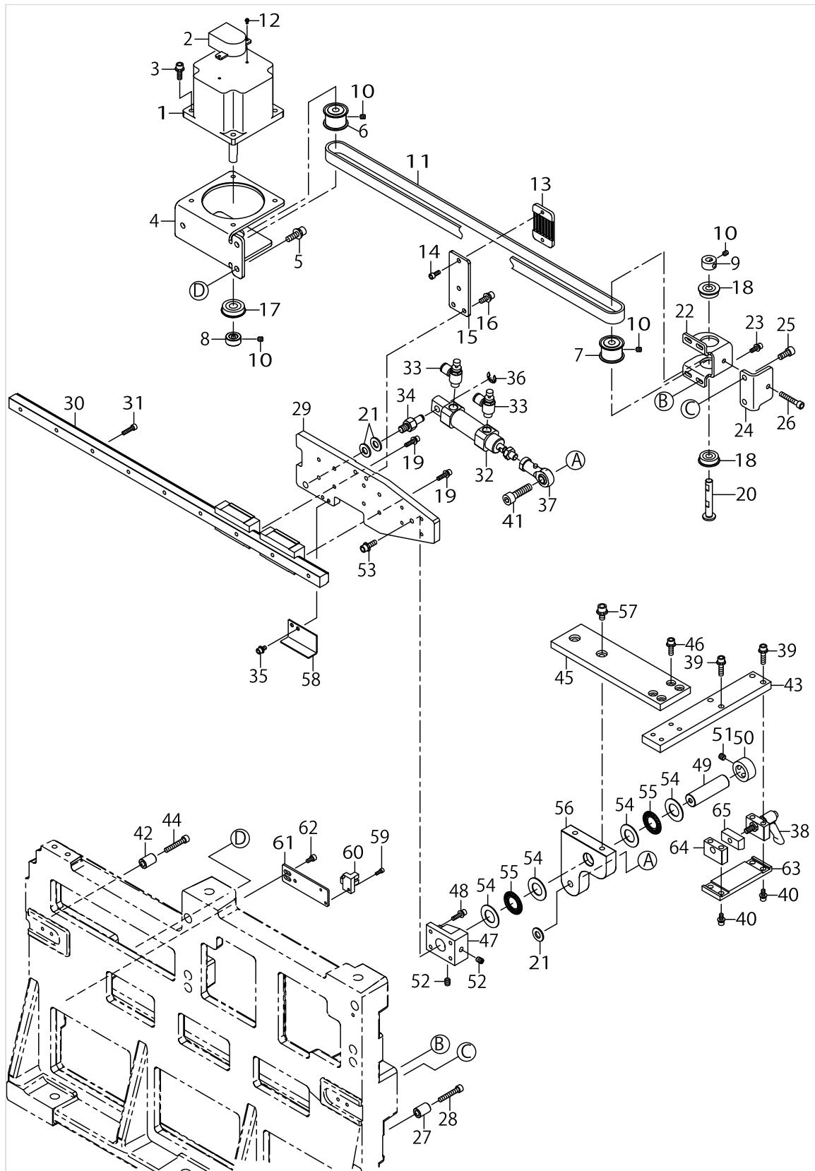
FORM PLATE MECHANISM COMPONENTS
