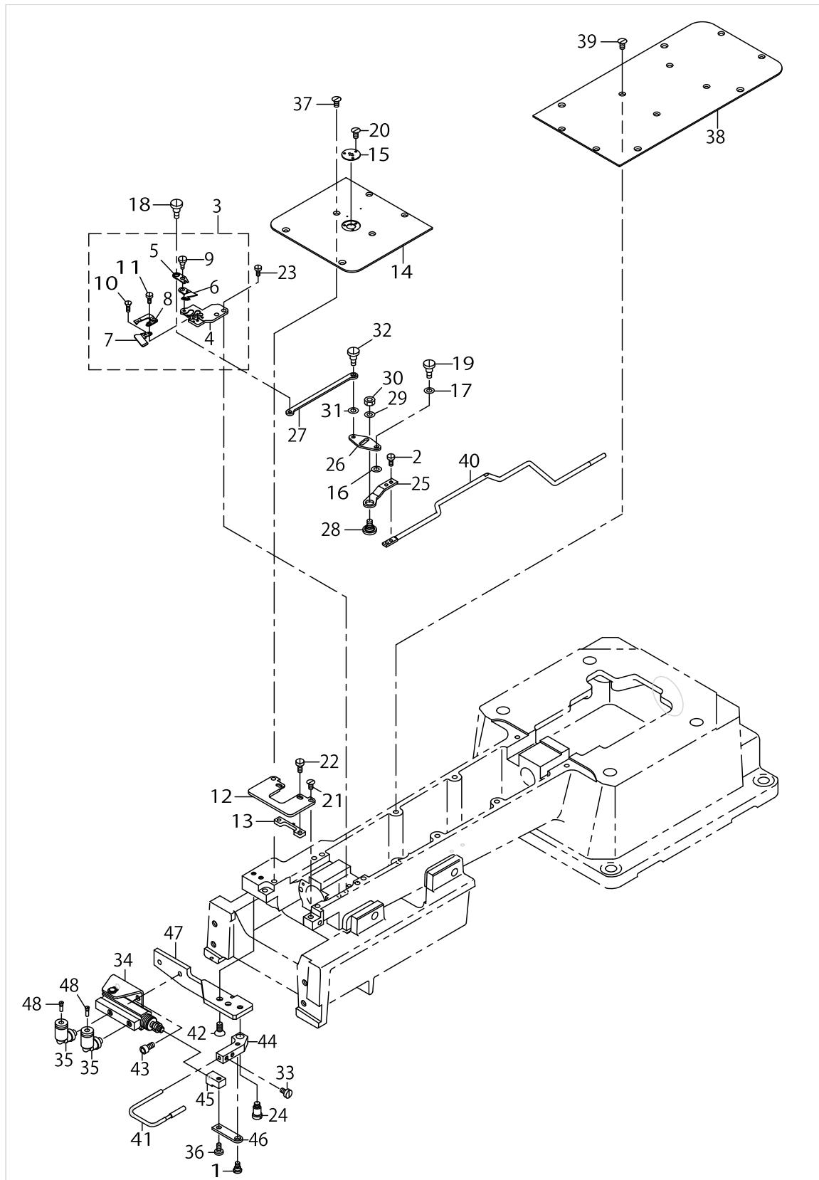
THREAD TRIMMER MECHANISM COMPONENTS (1)
