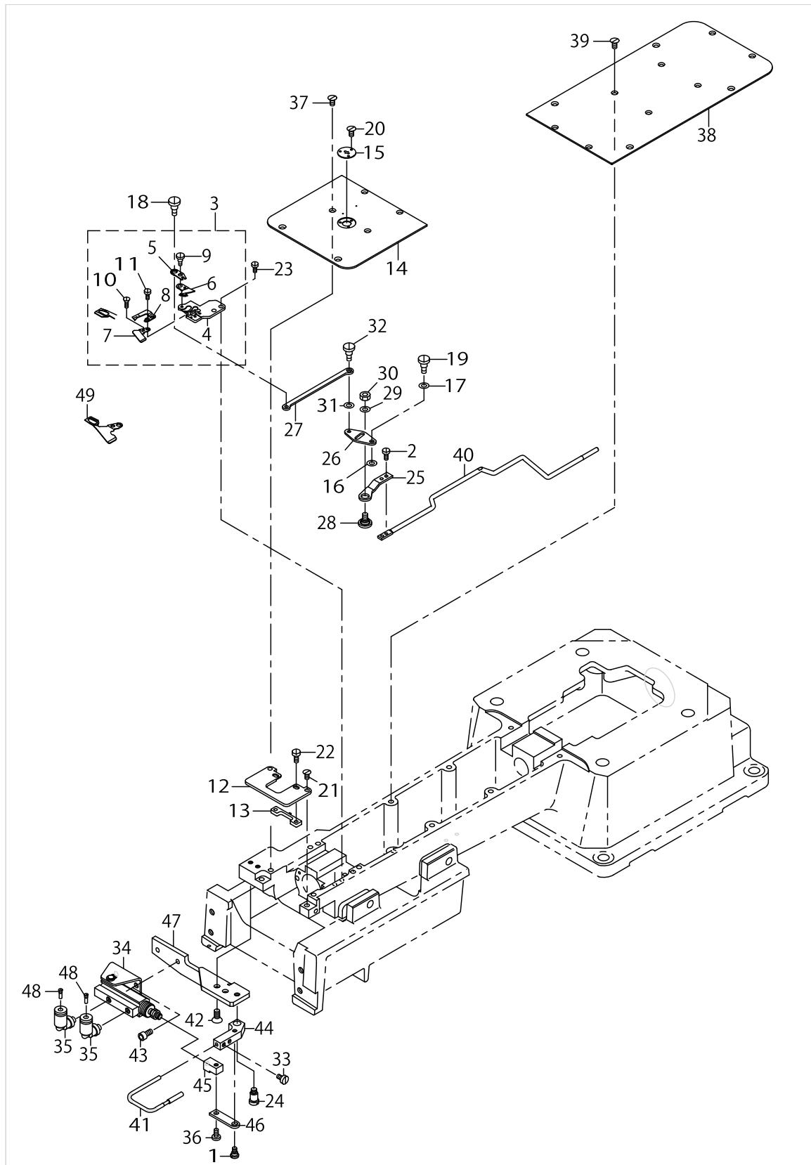
THREAD TRIMMER MECHANISM COMPONENTS (1)
