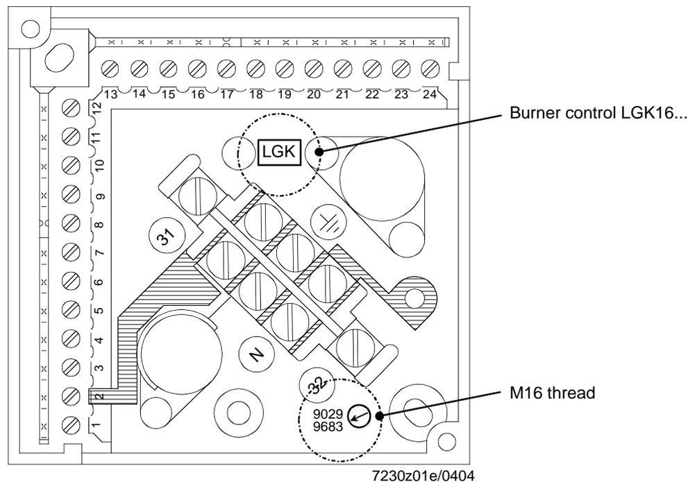
**Pg11** thread: Marked **9029** on the plug-in base (refer to «Dimensions»).
