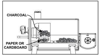
Once charcoal is lit, carefully pour the lit charcoal onto the charcoal tray closest to the intake damper. This will encourage the fire to burn and evenly. You can add unlit charcoal to increase the amount of fuel.
