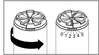
Adjust Roto-Draft<sup>™</sup> dampers using the included multi-tool.
